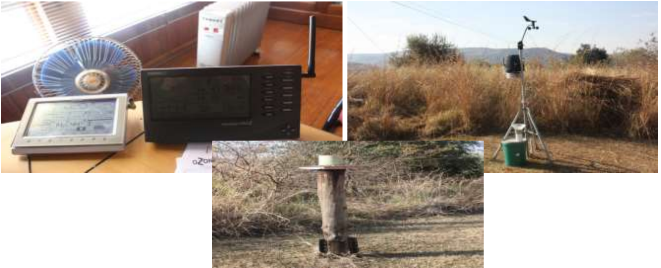
Figure 1: Shows equipment implemented at Cathedral Peak Didima to monitor climate variations – temperature, windspeed, rain, humidity. Data from the equipment is downloaded, stored for analysis of climate variations over time.
